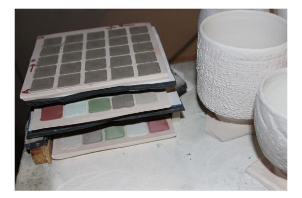
Another use of our "ice cube tray": colour tests with the use of drop counters We want to do color tests with oxide or dye in a given glaze. I made a video of this method https://youtu.be/NUAIc5UCCm4
